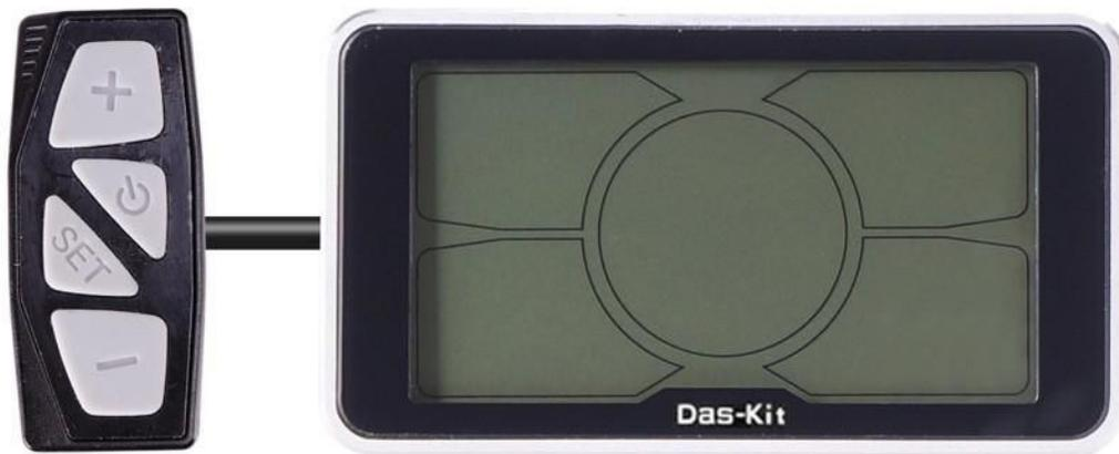
With the display on, the default indicators are riding speed, trip 2, PAS level, and battery indicator as shown in fig below. Press SET to switch the display information.
