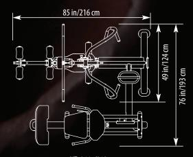
HT: 84 in/213 cm WT (Base Unit): 550 lb/249 kg WT (Leg Press): 190 lb/86 kg
