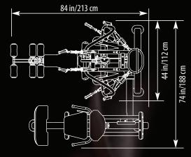
HT: 84 in/213 cm WT (Base Unit): 670 lb/304 kg WT (Leg Press): 190 lb/86 kg
